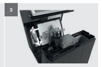
While holding the clamp away from the valve pull the valve towards you.
