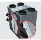
Remove the filters (and when present the pre-heater).
