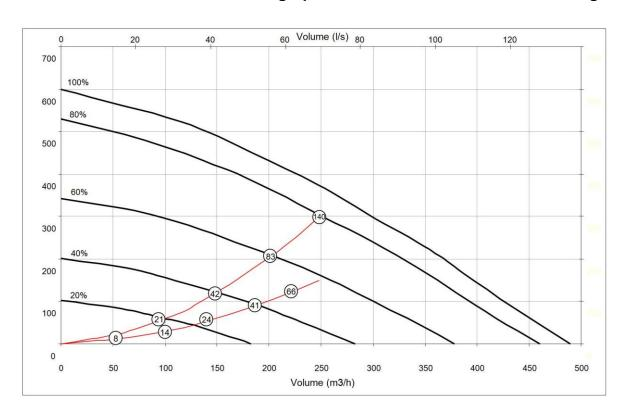
Note: Graph shows 2 typical system curves with total unit input power in Watts
