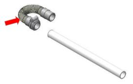
**6.** Fit pipe assembly into waste pipe and secure to condensate spigot with worm drive clip.
