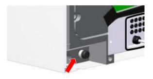
2. Remove the black Cap from the end of the condensate stub at the rear of the unit.
