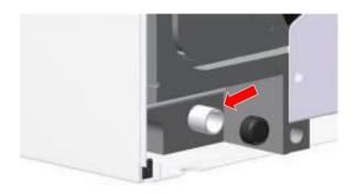
**3.** If not already fitted, fit the flexible condensate pipe and secure with worm drive clip
