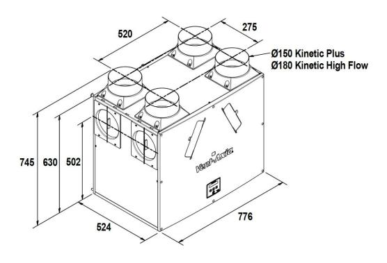
Figure 6: Sentinel Kinetic Plus and Sentinel Kinetic High Flow Dimensions
