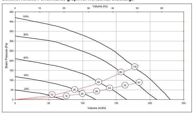
Note: Graphs show 2 typical system curves with total unit input power in Watts.
