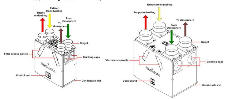
Fig 1: Sentinel Kinetic Right handed
