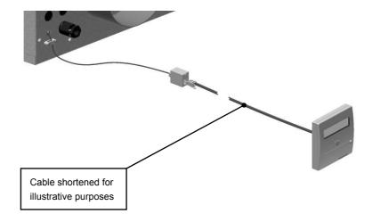
**3.** Connect the cable assembly to the Remote Control terminal block (the terminal block is colour coded to match the individual coloured cables and mount onto a single gang recessed wall box with the 2 screws provided.
