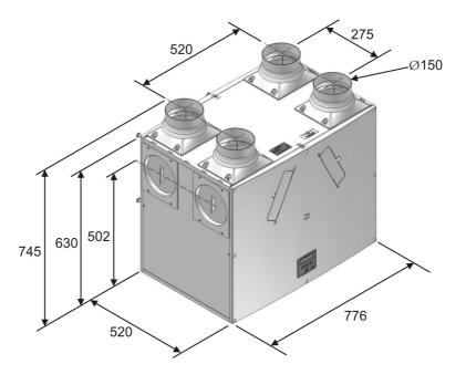
Figure 4: Sentinel Kinetic Plus Dimensions
