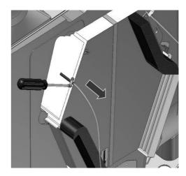
4. Pull out the cell and make sure that the rear bottom of the cell is securely resting on the lower edge of the foam so you can access the rear pressure tube. Repeat step 3 to detach the rear pressure tube. When the rear pressure tube is removed then the cell is free to clean.
