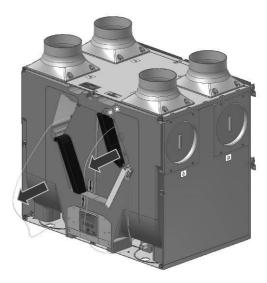
3. Pull out the Heat Exchanger Cell to gain access to the 2 screws on the cell as shown opposite. Loosen up the both screws (no need to remove them completely) to be able to remove the pressure tube and its rubber grommet strip.
