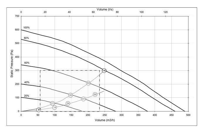
Note: Graph shows 2 typical system curves with total unit input power in Watts and the shaded area of the graph shows constant volume operation (CVP only).
