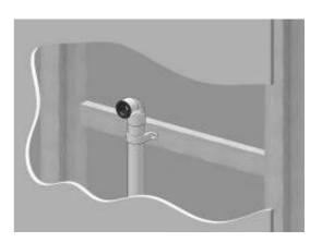
Fit the flexible condensate pipe to a 22mm diameter x 280mm long condensate pipe with worm drive clip.
