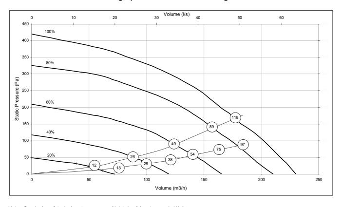
${\it Note: Graph show 2 typical system curves with total unit input power in Watts.}$
