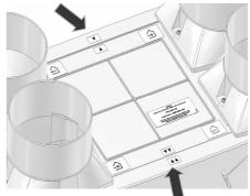
The arrow labels on the top edge of the Covers should be correctly matched to the arrow labels on the top of the Case.
