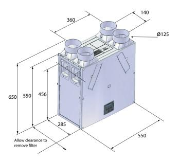
Figure 3: Sentinel Kinetic Dimensions
