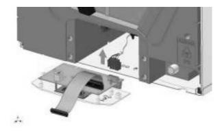
8. Remove the 2 screws and detach the rear Cable Inlet Plate.
