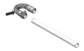
Fit pipe assembly into waste pipe and secure to condensate spigot with worm drive clip.
