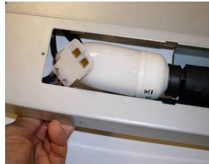
Figure 9: Passing cable through
