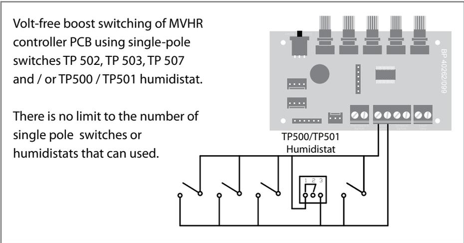
Boost switching and Humidistat connection ref EE 142
