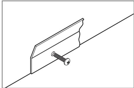
5. Fix the remaining Mounting Bracket to the unit using the M6 screws and washers provided, ensuring the interlock side is at the bottom. Do not overtighten
