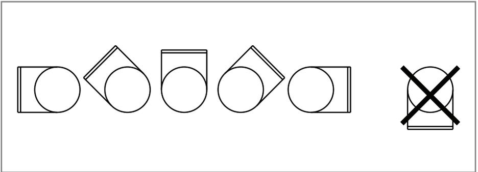
Duct Heater fitting orientation
