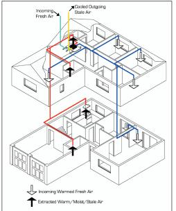
The system is designed to run continuously and should NOT be switched off except for maintenance or filter replacement. It is important to follow the
