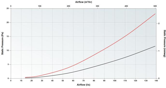
— Zehnder ComfoPipe Plus ø 160 mm, 45° bend — 2 x Zehnder ComfoPipe Plus ø 160 mm, 45° bend
