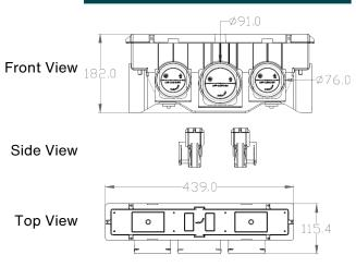
For use with Lamina/Bilamina/ComfoGrid Linea 400 slot diffusers
