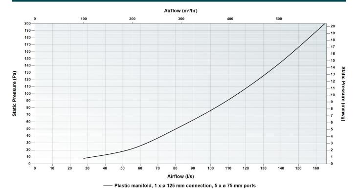
For use with Zehnder ComfoTube ø 75 mm semi-rigid ductwork
